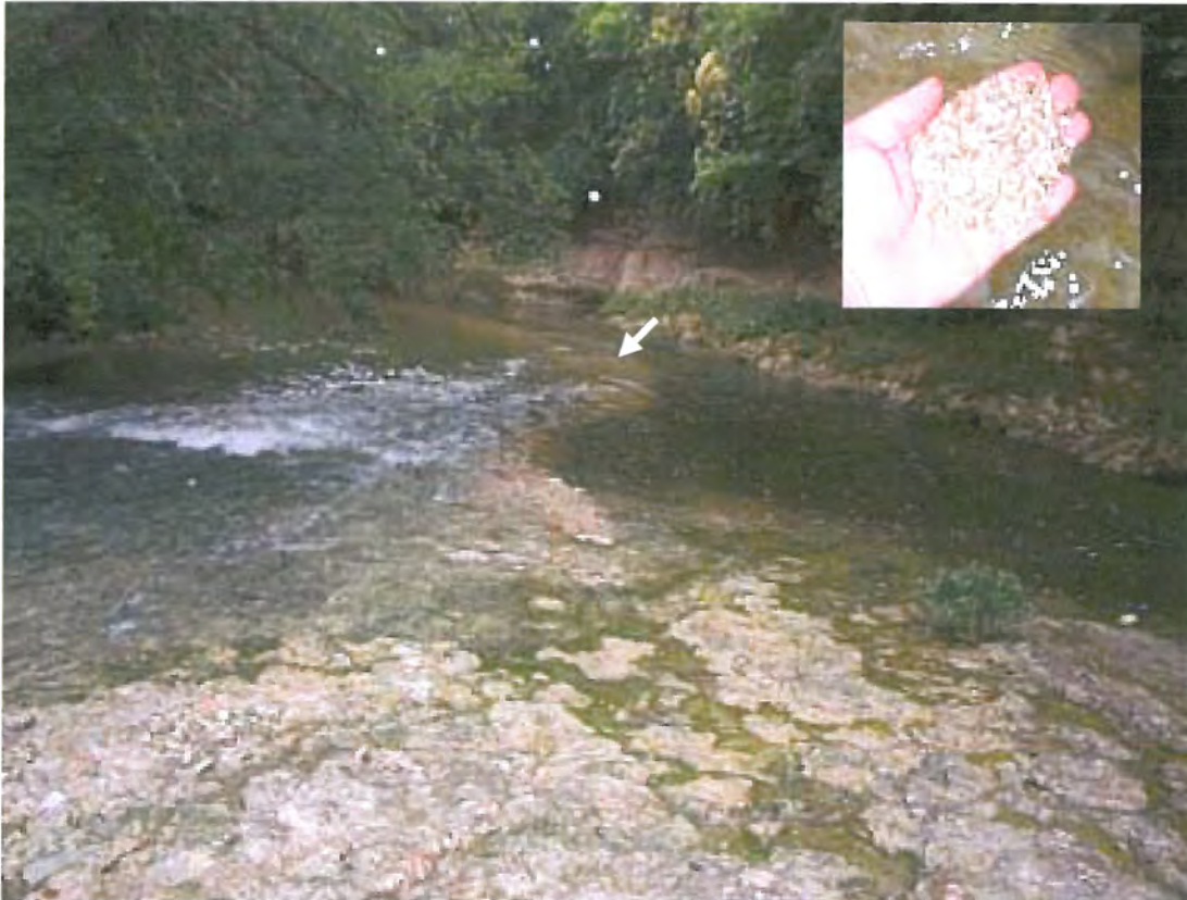
The white arrow indicates a bed of deposited sediment where the effluent and stream flow meet. This sediment consists almost entirely of gravel. Areas 1/4 mile upstream and downstream contained a slightly higher content of fine sands, but gravel consistently accounts for the majority of the sediment.
