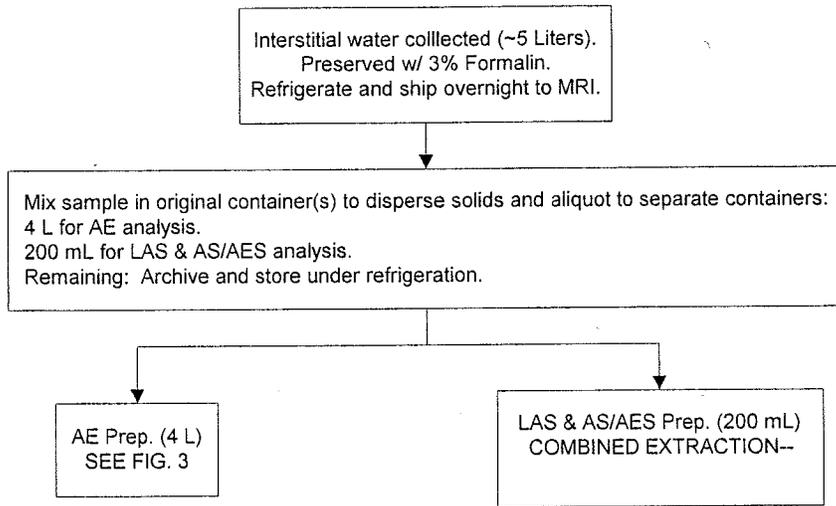
FIGURE 1. INTERSTITIAL WATER PROCESSING
