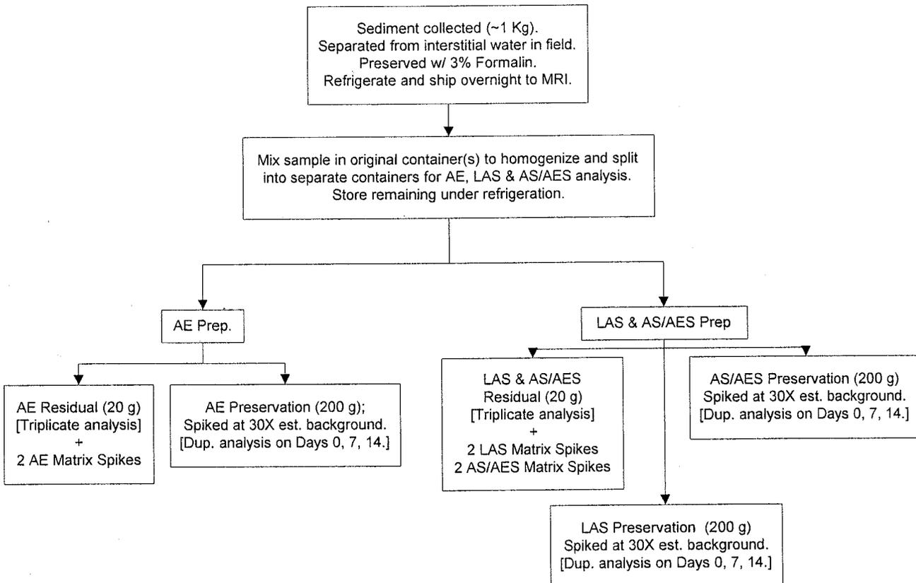
FIGURE 3. EXTRACTION / BREAKTHROUGH DETERMINATION
