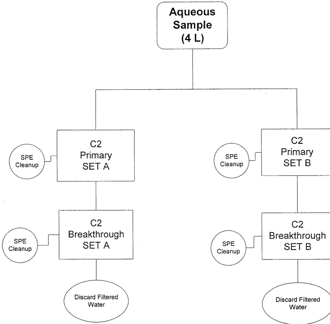
**Extraction of Interstitial Water using C2 Cartridge:**
