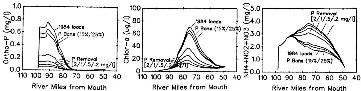
Figure 2. Effect of phosphorus control on water quality
